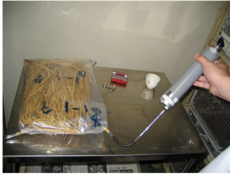
Fig.1-2 Determination of ammonia gas emission with Kitagawa Precision gas detector tubes.
